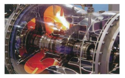
When gas turbines are run, they become foul with airborne contaminants such as oil, soot, unburned fuel, soils and salt which encrust compressor components. Power loss follows as the compressor loses efficiency and degrades the performance of the engine, leading to higher operating temperatures, increased fuel consumption and shorter component life.
